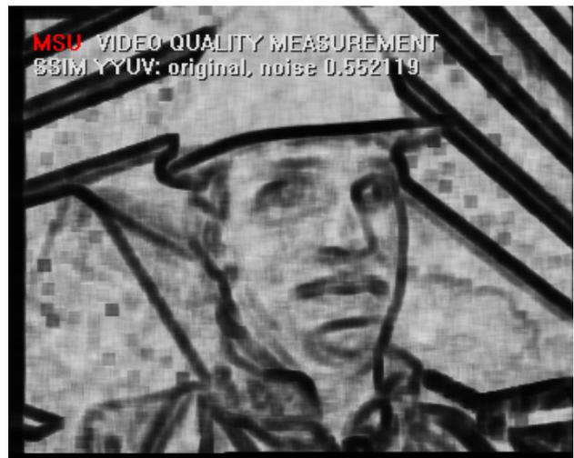
(b) SSIM map for noisy image, **SSIM = 0.552119**
