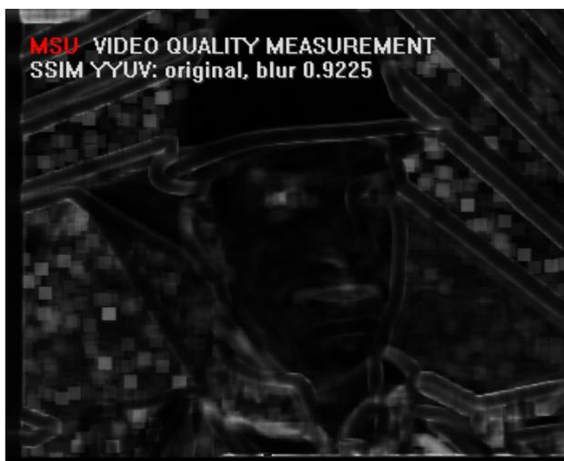
(c) SSIM map for blurred image, **SSIM = 0.9225**
